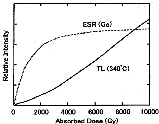
Fig. 4. TL and ESR growth curves of quartz phenocrysts.
